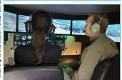
**Aviation Training Device (ATD)** – A replica of aircraft instruments, equipment, panels, and controls in an open flight deck area or an enclosed aircraft cockpit. It includes the equipment and computer programs necessary to represent aircraft (or set of aircraft) operations in ground and flight conditions having the full range of capabilities of the systems installed in the device as described in AC 61-136 for a specific Basic or Advanced qualification level.
