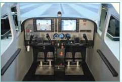
Flight Training Device (FTD) – A replica of aircraft instruments, equipment, panels, and controls in an open flight deck area or an enclosed aircraft cockpit. It includes the equipment and computer programs necessary to represent aircraft (or set of aircraft) operations in ground and flight conditions having the full range of capabilities of the systems installed in the device as described in 14 CFR part 60 and the Qualification Performance Standard (QPS) for a specific FTD qualification level.
